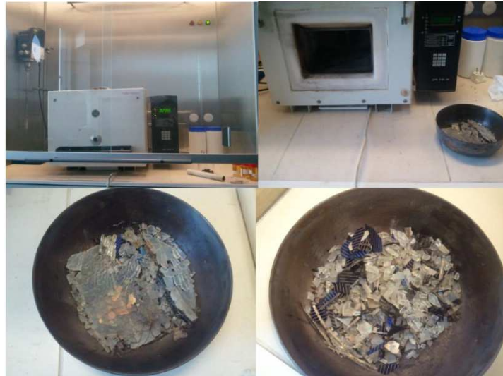
Fig. 7. Heat treatment of PV modules.
