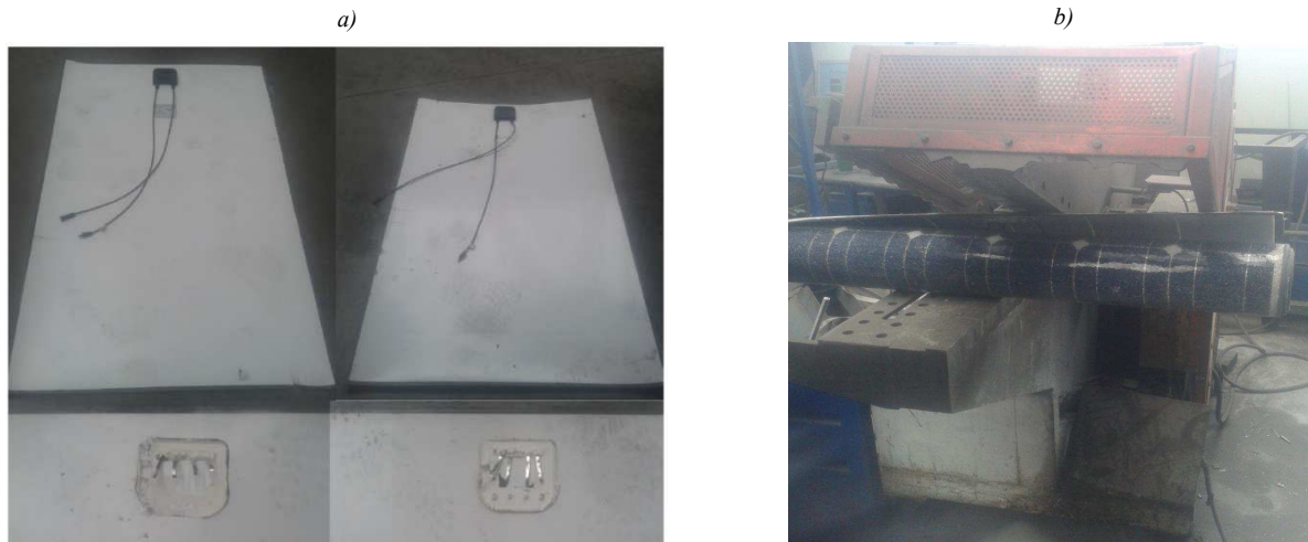
Fig. 10. a) Removed aluminium frames and junction boxes, b) PV modules cutting into two halves.
