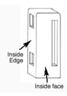
**1.** On the inside (3/4") edge, make a rout that is 1/4" deep and 1/2" wide that runs from 1/2" from the top of the leg to 2 1/2" from the top. This rout should be 1/8" in from each side. This slot will accommodate the top support that runs along the length of the rack.
